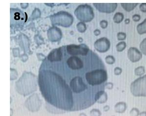
For example, condensation contamination (Figure-8) is created by temperature differentials of surfaces passed from one ambient to another: service truck in winter weather to an inside data center.
