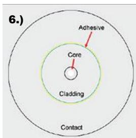
Figure-6 is the customary view of a fiber optic end face. It is a limited two-dimensional perspective of ~250 microns. There are 2500 microns on a 2.5mm surface, thus considerable surface area is not characterized on the ‘horizontal’ and completely disregarded on ‘vertical’ and other ‘intersurfaces’.
