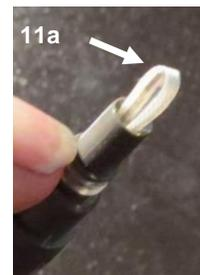
Notice the swab tip in Figure 10b is ‘folded’: the design compensates for UPC and APC configuration. Swab tools are used in high-tech wafer fabs and medical applications. Don’t be allured by ‘convenience-for-convenience’s-sake’! Seek tools that perform in applications specific methods and procedures. I urge you: request samples and factory support when you have having a ‘tough dog problem’ that does not seem to resolve by changing brands!
