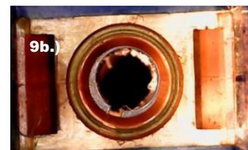
Secondary Contamination may be exacerbated by adding debris from an alignment sleeve. (Figure 9b). The realities of cross-contamination underscore the need for inspection of not only both connector surfaces, but also alignment components. Views of a contaminated adapter and alignment sleeve were not possible until this time.
