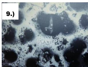
While the fluid on this "primary surface" image is obvious, as well is obvious condensation extending outside the 400x field of view. Fluids located outside the field-of-view can leech into active transmission zones in the time of post cleaning and post inspection. "Best Practice" is to consider all surfaces at time-of-service.
