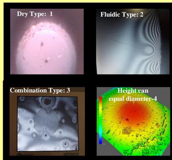
Existing standards for end face inspection limit the field of view to zones within a two-dimensional field-of-view limited to (video) magnification ranging between 100x-400x usually measured at 250-300 $\mu$ m radius of the core. By these standards, the end face is divided into three or four “zones”, all contained on the horizontal axis. Of course, a connection is a three
