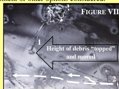
Dry cleaning a complex debris has several significant limitations. Among those is the possibility of ESA attraction but more significantly is the reality that drying cleaning tends to move and not remove debris and contamination. The image (FIGURE VII) shows two aspects of dry cleaning: 1.) debris has height and 2.) the process moves debris. Dry cleaning may be effective on an oily contamination; this is dependent on the wiping material within the dry device itself.
