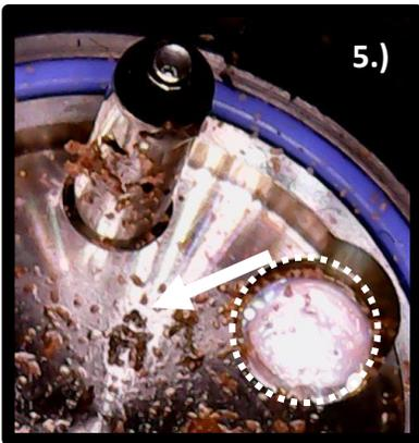
In the expanded beam images (5/6.) most typically the expanded beam manufacturer would be concerned with the lens (white circle, image bottom left). However, clearly there is also contamination on the alignment pin and inter-surfaces. These can migrate.
