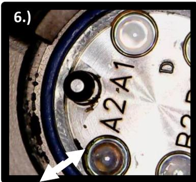
Contamination on the adapter housing of a SC connector (7.) can transfer either with a touch-insertion
