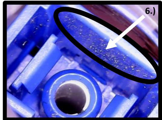
'jumper to backplane', or also in the time of post cleaning and post inspection. Knowing the physical location of these 'soil points' is important to successful high speed and high capacity installations. Utilizing a rotating adapter device can eliminate multiple cleaning, return of soiled components as 'defective-warranty', and enable the technician to concentrate on far more technical matters than improper cleaning and limited inspection
