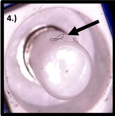
For 'large can' expanded beam, TFOCA, or other such style connectors with 2-4-8-12 or more fibers, the rotating adapter clearly sees each lens, but also 'inter-surfaces' and debris at various points that can be 'contamination points'. For both commonly used SC, LC, MT-Type, and even old-style "biconic connectors, the technician views and isolates contaminated surfaces that can create a fouled "Zone-1" fiber core. Image 4 shows a thread on the 'vertical ferrule'.
